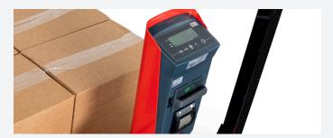
**Thermal printing capability** provides load details, including date, time, counted pieces, gross/net weight, and total weight.
