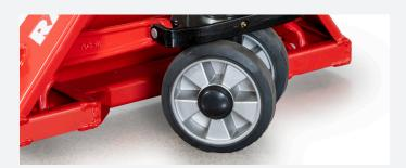
**Polyurethane steer wheels and load rollers** provide smoother, more comfortable operation.
